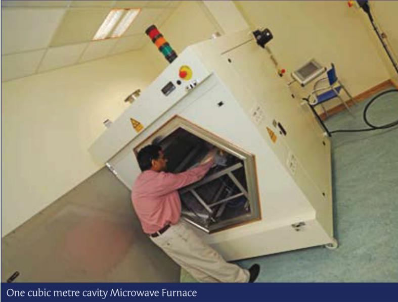
One cubic metre cavity Microwave Furnace
